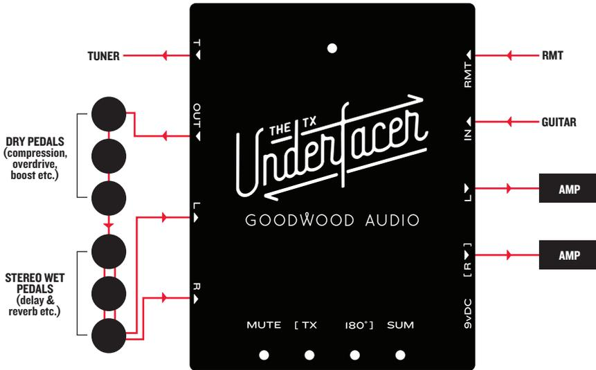
If you have a vintage fuzz or wah, or any pedal that doesn't like being after a buffer, plug directly into that pedal, and from there go to the input of The Underfacer.
